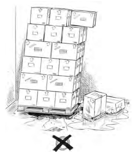
Figure 9. Tipping Pallet Due to Un-level Floor
