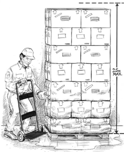
Figure 11. Example of Crushed Boxes Due to High Stacking
